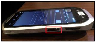
Pressing and holding either one of these buttons will activate the barcode-scanning function: a red-light, cross-hair projection from the top edge of the scanner. Aiming these cross-hairs at the center of a ticket's barcode (or QR code), at a distance of about three inches, should generate a response message on the lower portion of the scanner's screen (as well as an audible beep/chime).
